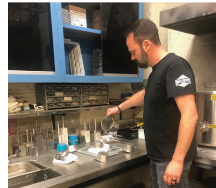
Pouring Cerrobend for a custom electron cut out for radiation therapy.
