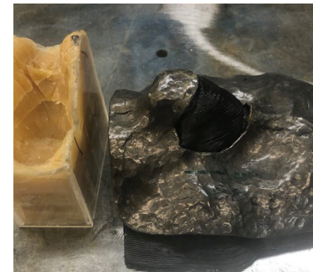
A radiation shield mask made from resin and beeswax, with hammered lead using a 3D printed ABS replica of a facial model.
